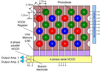
Figure 1. The block diagram of developed sensor
