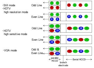
Figure 4. The output signal sequence
