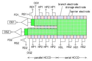
Figure 2. The schematic diagram around the branch electrode
