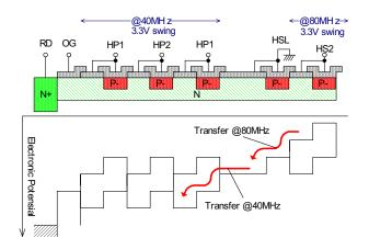
Figure 3. The cross section around the branch electrode
