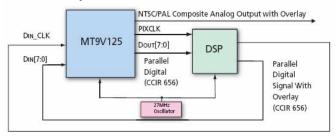
Figure 4: Typical Usage Configuration with Overlay
