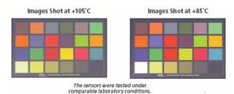
Figure 2: Sensor Performance at High Temperatures
